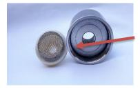
Separator head - removable screen of coarse dirt.
